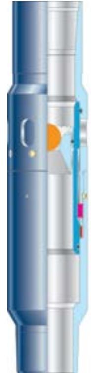
*The Falcon ball-actuated frac valve consists of balls that seat in the valve and allow the frac sleeve to open as pressure increases. Options for a single- or multiple-ball seat are available to suit the number of zones to be fractured.*
