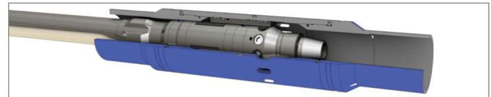
**Stage 4.** The CT string loses tension, indicating that the sleeve has shifted and the tool can be pulled through the sleeve cavity. If a sleeve is partly shifted, the keys will retract only after the operator stops pumping and releases the hydraulic differential pressure.
