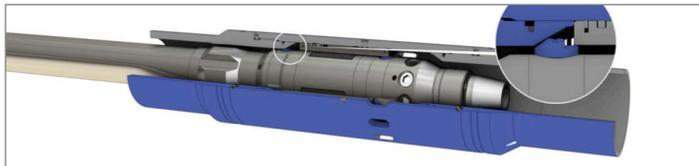
**Stage 3.** When the sleeve is fully actuated (100% open), the leading keys reach a kickoff profile in the upper sleeve cavity, retracting all the keys and releasing the sleeve.
