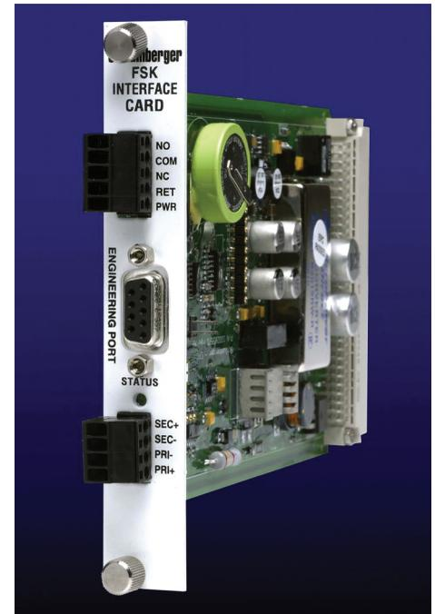
*The FIC NG supports all FSK gauges used with WellWatcher permanent monitoring systems.*
