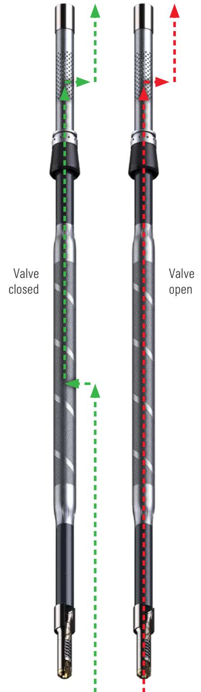
*This configuration is used when the PumpGuard assembly is suspended with a cup packer below an ESP or rod lift pump. Green and red arrows indicate fluid flow paths when the pressure-activated valve is closed and open, respectively.*
