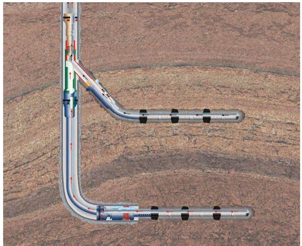
RapidX TAML5 high-strength, hydraulic-sealed multilateral junction.
