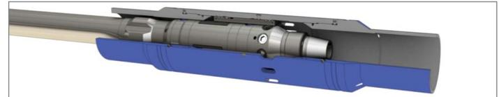
**Stage 4.** The CT string loses tension, indicating that the sleeve has shifted and the tool can be pulled through the sleeve cavity. If a sleeve is partly shifted, the keys will retract only after the operator stops pumping and releases the hydraulic differential pressure.
