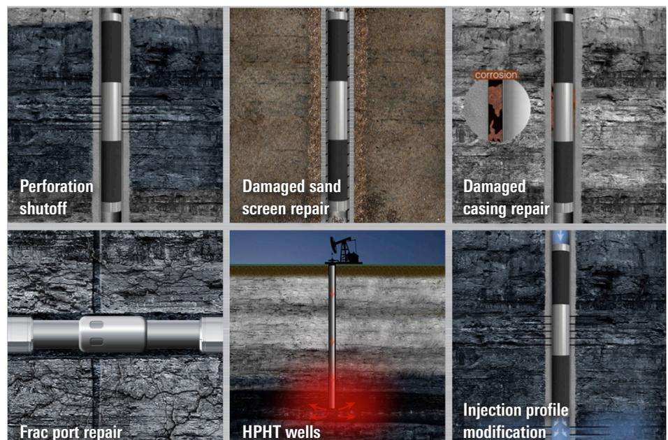
*Saltel expandable steel patches provide a reliable, permanent solution for many repair and remedial operations.*
