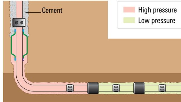
0-1 packer: Off-bottom cement above a high-pressure hydraulic fracturing completion.
