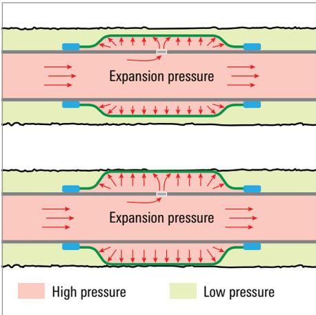
Setting process for the 0-0 model of the packer.
