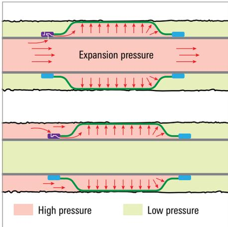
Upper image: Setting process for the 1-0 model of the packer (similar to the process for the 0-1 model). Lower image: Subsequent pressure balancing of the high-pressure annulus and the packer chamber, enabling the packer to maintain an effective seal.
