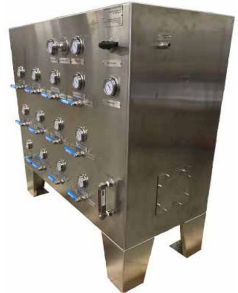
Surface hydraulic control system, comprising a hydraulic power unit and an integrated hydraulic manifold unit.
