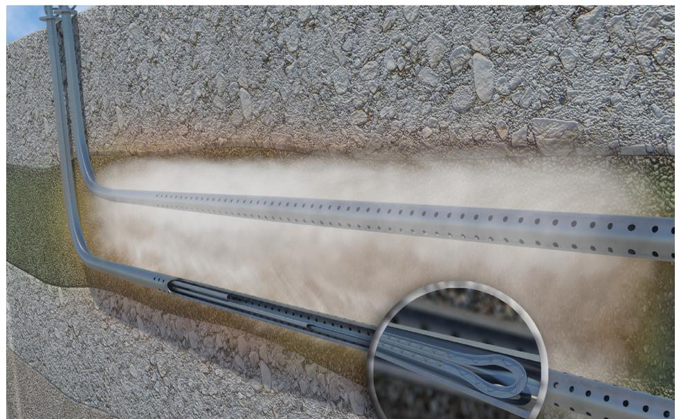
*The WellWatcher BriteBlue HT high-temperature multimode DTS fiber, installed in a heavy-oil thermal recovery application, is pumped in and through a conduit located inside a coiled tubing string using Schlumberger patented techniques. The coiled tubing is hung from the surface across the producing interval, and the temperature of the entire well is monitored to ensure that the correct level of subcooling is maintained to avoid steam breakthrough from the injector above.*
