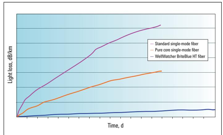
*The WellWatcher BriteBlue HT high-temperature multimode DTS fiber transmits more light than conventional single-mode fibers when interrogated by a distributed-temperature acquisition unit in harsh, accelerated test conditions: 250 degC [482 degF], 3,447 kPa [500 psi], and high levels of hydrogen.*
