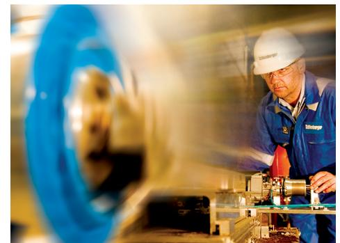
*Schlumberger offers multiple means of deploying a fiber into a wellbore, including fiber pumping, fiber-optic cable, and hybrid optoelectric cable. Shown is the deployment beam used for fiber pumping.*
