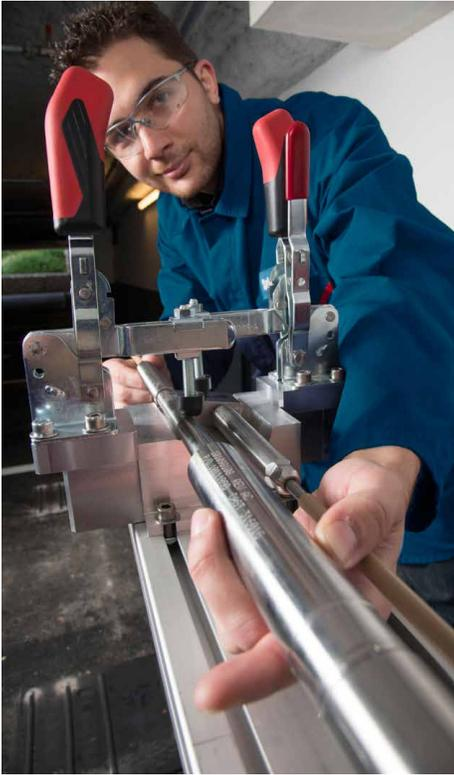
The WellWatcher Flux system station is inspected in a vice during manufacturing.
