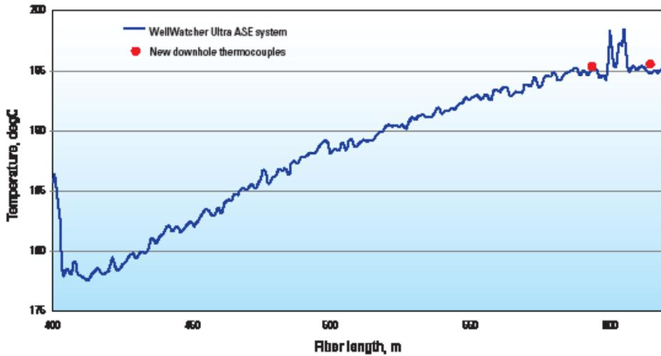
This temperature profile, acquired with the WellWatcher Ultra ASE DTS system, shows that after the system corrected for the error induced from a degraded fiber, its measurements agreed with two independent reference points obtained from newly installed downhole thermocouples.
