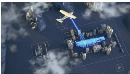
**Fig. 3.** Positioning multiple IoT-enabled sensors on large field sites can detect airborne methane, triangulate to the leak location, quantify the emission rate and alert the operator.
