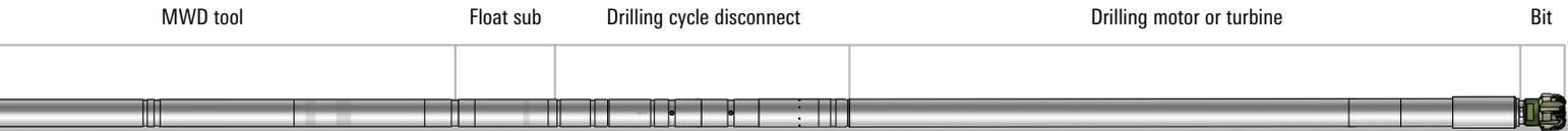
*The CTDirect system BHA enables better steering based on direction and inclination, gamma ray, annular-pressure-while-drilling, and internal-pressure-while-drilling measurements.*
