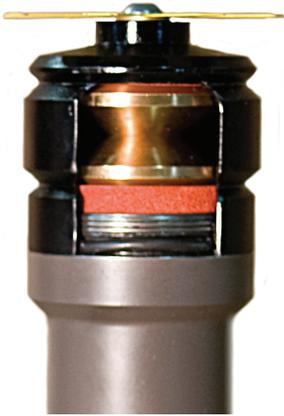
*The PowerCutter tubular cutter explosive charge (shown in cutout section) produces a 360° radial explosive jet.*
