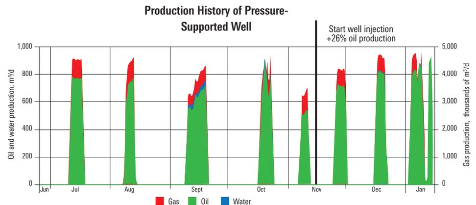
After the ACTive system operations improved the efficiency of an injector well, oil production in nearby wells increased by 26%.
