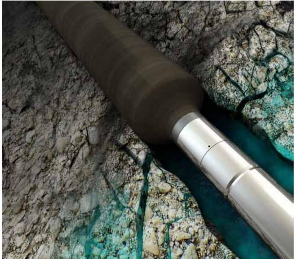
*The CoilFLATE through-tubing inflatable packer distributes the anchoring force over a large surface area. Thus, no damage was done to the fiberglass coating of the well's casing.*
