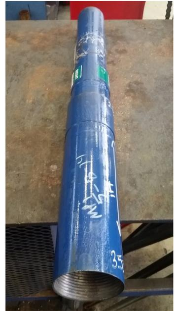
*A box tap with a tapered OD was used to successfully fish the valve from the well.*
