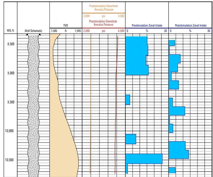
Comparison of pre- and poststimulation injection profiling along the openhole horizontal section. The acid stimulation targeted the middle section and resulted in a more uniform water injection distribution along the open hole. Surface injection pressure was reduced from 1,000 to 0 psi.
