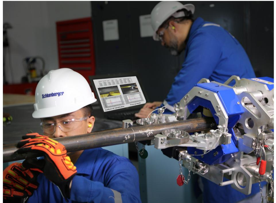
*Schlumberger uses a novel CT inspection approach based on MFL interpretation to assess mechanical defects. This approach does not depend on manual measurements of the dimensions of CT anomalies, thereby allowing consistent, automated, in real-time inspection assessment.*
