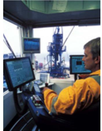
*The CT SEAS unit offers an ergonomically designed cabin which enhances operator control while reducing personnel requirements, rig-up time, and costs.*
