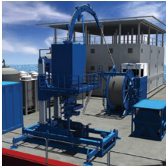
*The CT SEAS unit only has 10 primary skids, which cuts crane lifts off the boat to 36 from 53 in typical operations.*
