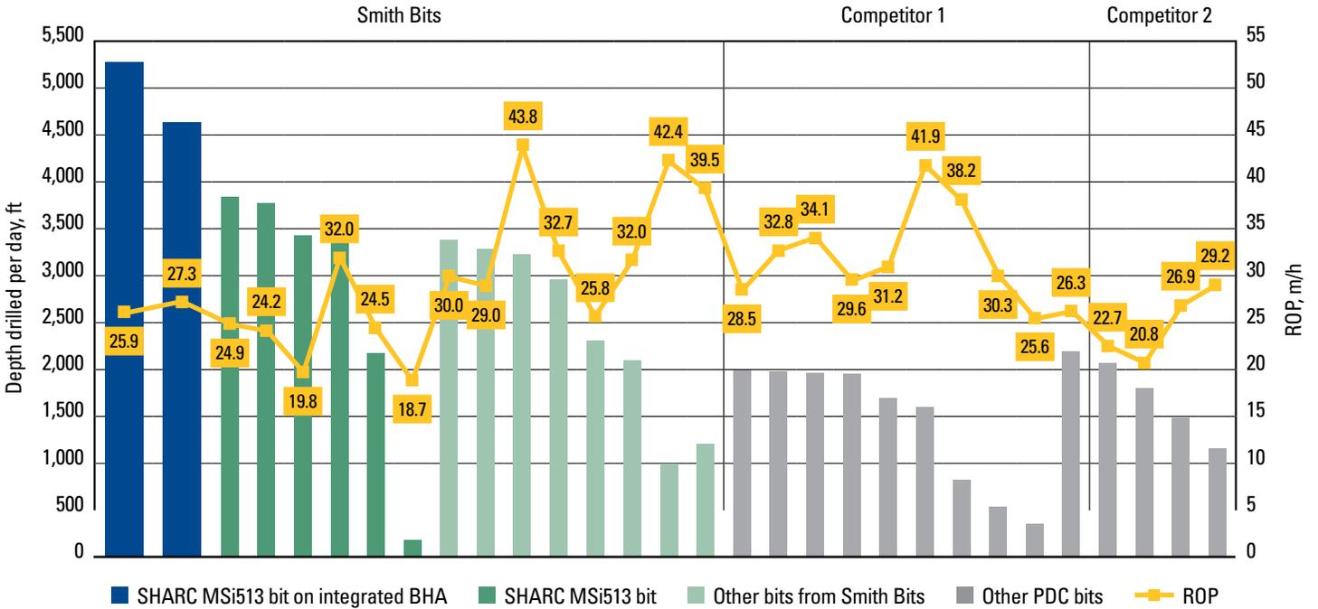
When compared with offset drilling performances using conventional PDC bits (gray) and SHARC MSi518 bits run on conventional BHAs (green), the number of feet drilled per day increased significantly using the SHARC bit run on the specially engineered drilling system (blue) that combined a suite of Schlumberger technologies and services.
