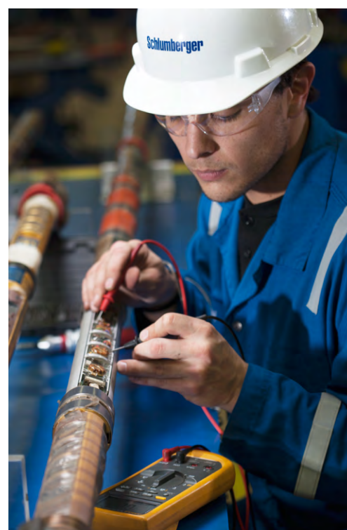
DigiScope service acquires real-time measurements for drilling optimization and formation evaluation.
