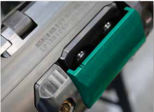
PowerDrive Orbit system, with its newly developed pad design and self-steering automation, helped improve ROP and drill from 4,085 to 4,704 m while keeping verticality of the well within 0.5 degrees.
