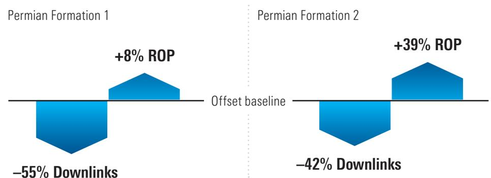
*Auto-curve reduced downlinks to the RSS 42% and 55% in the curves of two different Permian Basin fields. The responsiveness of the autonomous downhole controls improved performance, including increased ROP in all 14 wells.*
