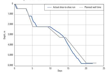
The DynaForce motor and PowerDrive Orbit G2 RSS enabled Vista Oil & Gas to drill shoe to shoe in a single run in an interbedded formation and saved 2 days from original planned well time.
