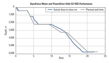
The DynaForce motor and PowerDrive Orbit G2 RSS enabled Vista Oil & Gas to drill shoe to shoe in a single run in an interbedded formation and saved 2 days from original planned well time.
