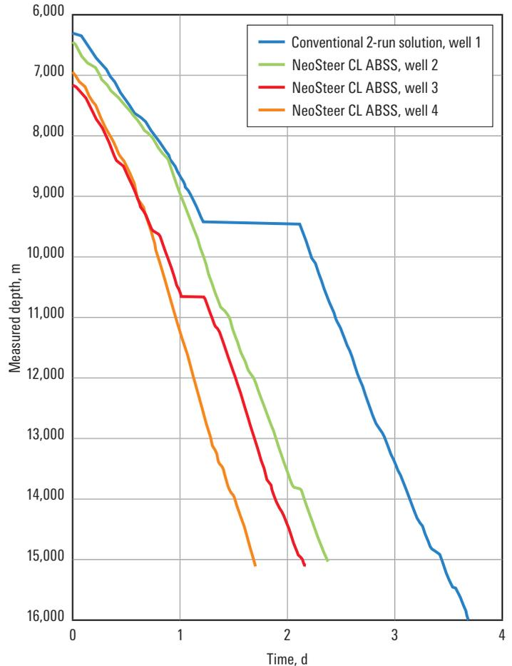
*After fine-tuning the NeoSteer CL ABSS performance, Repsol saved roughly 2 days on the last well alone, compared with the time it would have taken to drill the well with a conventional BHA.*
