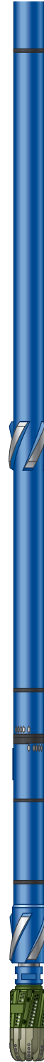
Stabilizers helped the Neyfor turbodrill hold the planned inclination and azimuth throughout its 250-m run.
