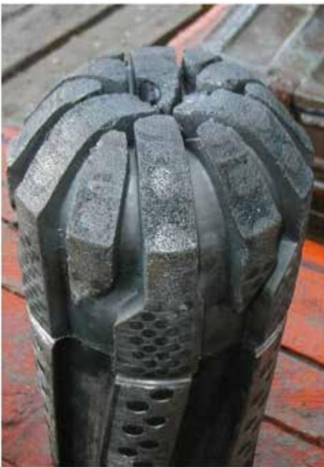
The Smith Bits Kinetic impreg bit set a new record with the longest single run through the Nikanassin. The next run utilized the same bit model to confirm the bits resistance to extreme wear while maintaining an acceptable ROP. †
