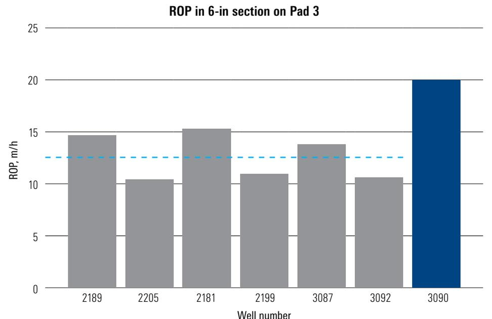
*The RSS drilled the challenging 6-in horizontal interval at an average ROP of 20 m/h—67% faster than the average ROP in offset wells.*
