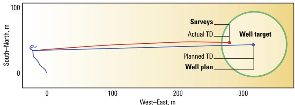
Push-the-bit trajectory control enabled drilling to section TD 5 days ahead of plan.
