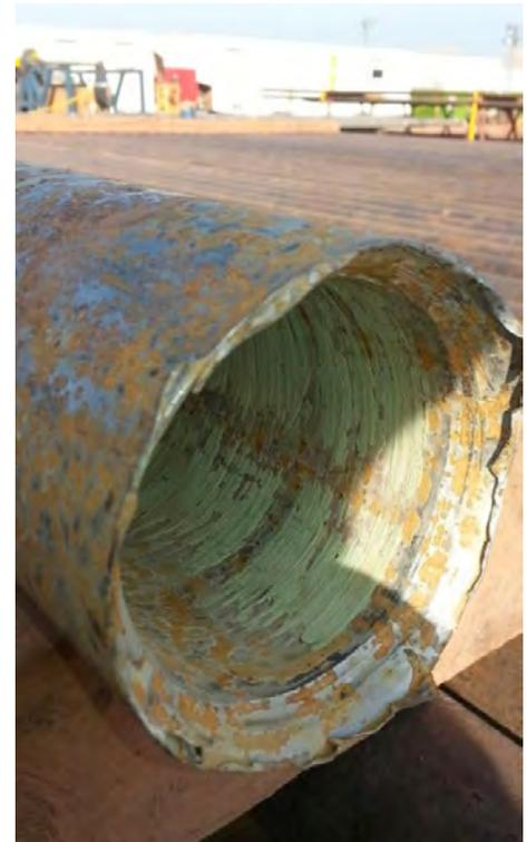
*Pacific Rubiales used the TT hydraulic pipe cutter to successfully sever the 4-in drillpipe below the shoe.*
