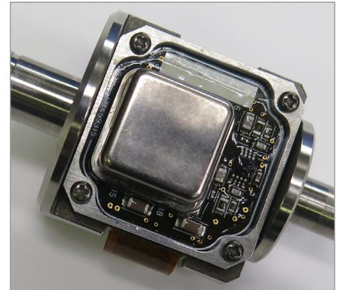
*Solid-state MEMS technology means the GyroSphere service can withstand the rigors of drilling operations, including shock and vibration.*
