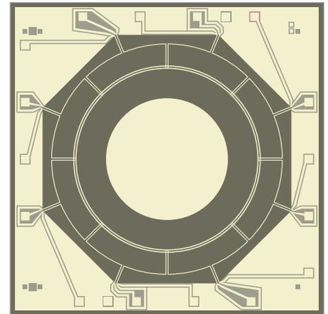
*The GyroSphere service uses an internal vibrating structure to ascertain planetary rotation relative to the sensor.*
