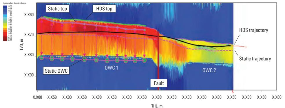
*An operator improved well path location in relation to reservoir fluids using the HDS service. When combined with reservoir-scale mapping from the GeoSphere service, the top and oil/water-contact (OWC) boundaries were further optimized.*
