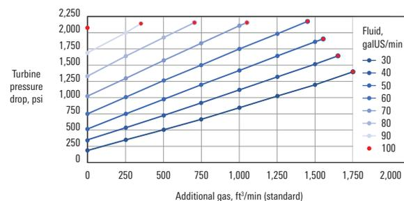
Values based on a reservoir pressure of 1,900 psi and temperature of 270 degF. The end of each curve represents the maximum additional gas for a given fluid flow rate.
