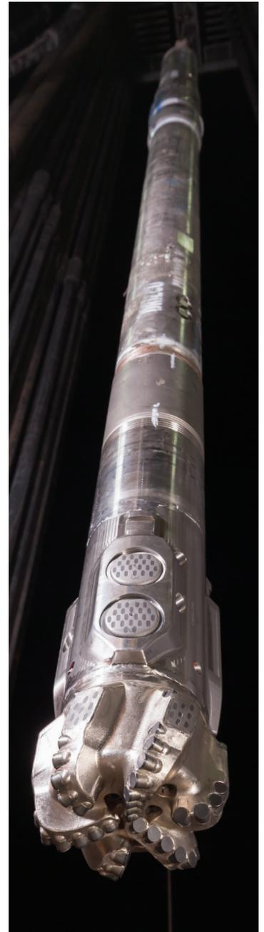
*With the PowerDrive xCL RSS, the pistons are located closer to the cutting structure for greater dogleg leverage in single-run, single-BHA applications.*
