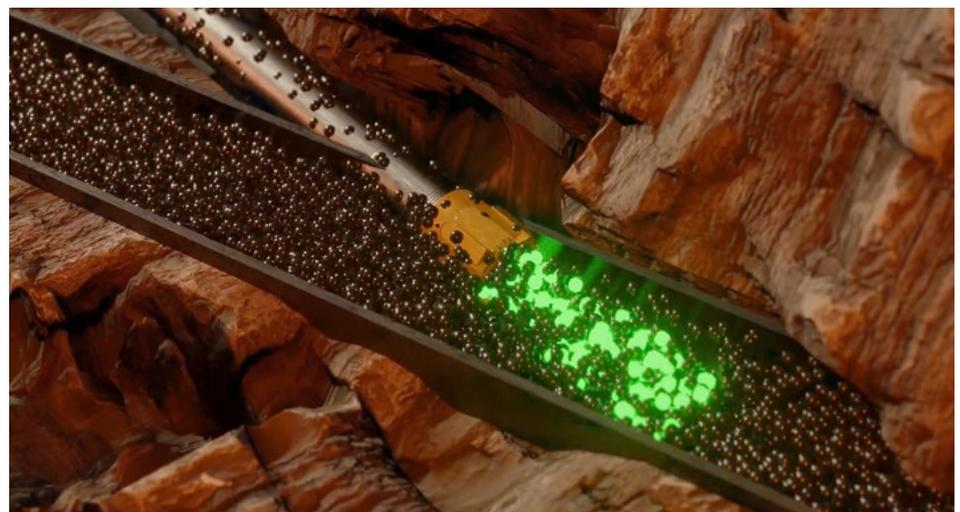
*K&M plans and monitors the drilling angle of a relief well to the target well intercept point. Well-killing operations subsequently begin by penetrating the target well and implementing dynamic kill parameters.*
