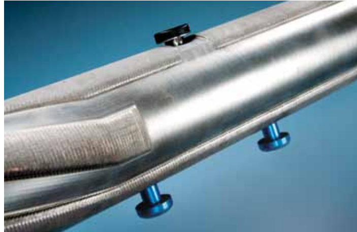
Two setting pistons—shearable and drillable—ensure perfect setting of this slimhole tool against the wellbore wall in any hole deviation, regardless of orientation.
