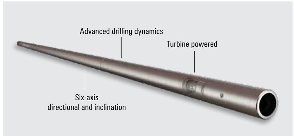
*The TruLink service uses a turbine-powered sub that provides reliable physical telemetry up to 20 bps. The six-axis directional and inclination delivers dynamic surveys while drilling.*
