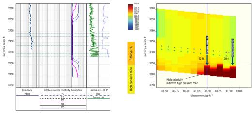
The IriSphere service enabled resistivity ahead of the bit detection 40 ft ahead of the tool and enabled geostopping between 20- to 40-ft MD before entering the high-pressure zone. Based on deep electromagnetic technology, the service was used to accurately pick up the top high-pressure zone ahead of the bit.
