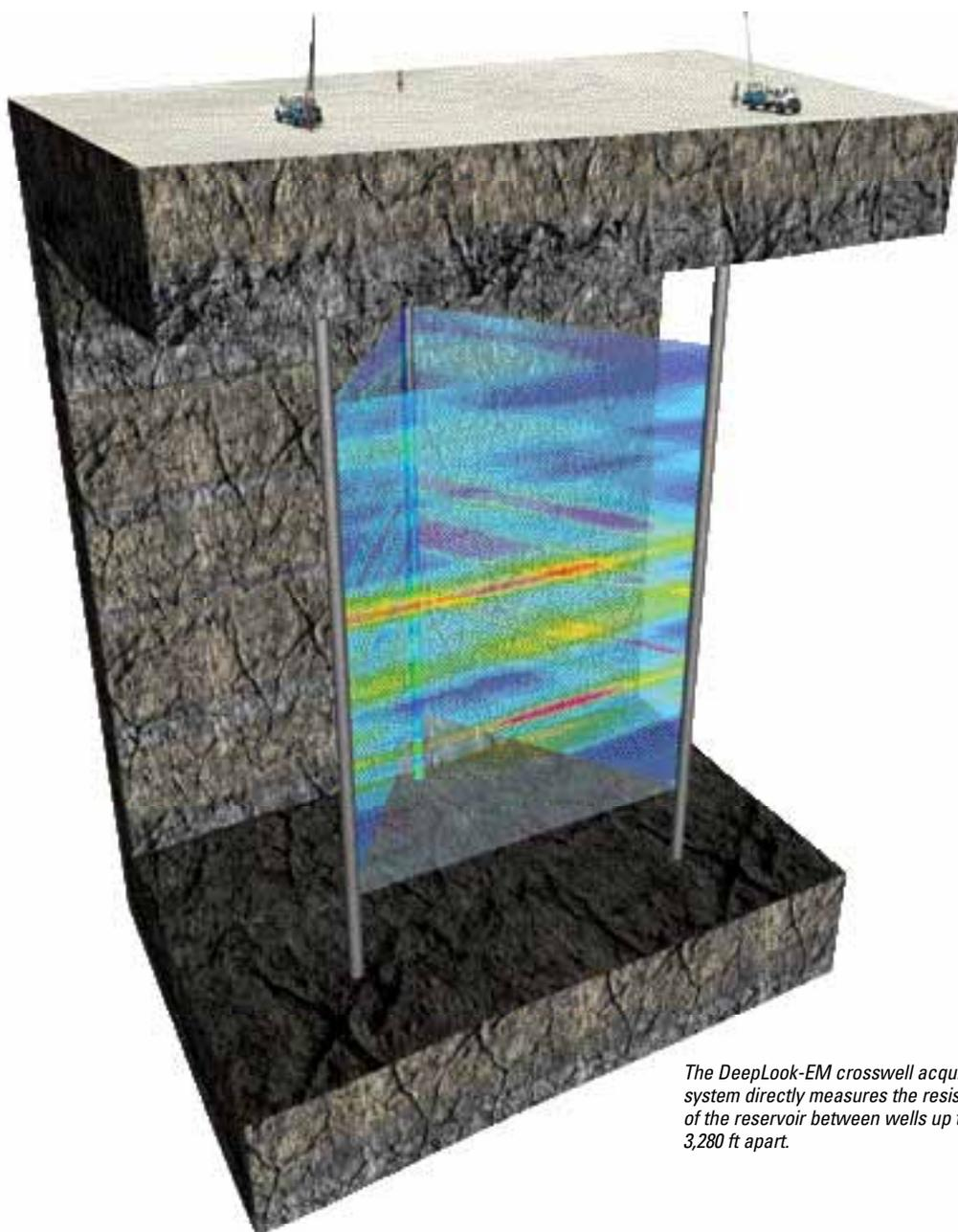
*The DeepLook-EM crosswell acquisition system directly measures the resistivity of the reservoir between wells up to 3,280 ft apart.*
