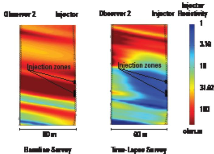
The DeepLook-EM images after water injection confirm that large volumes of water are swept within and outside of the injection interval.
