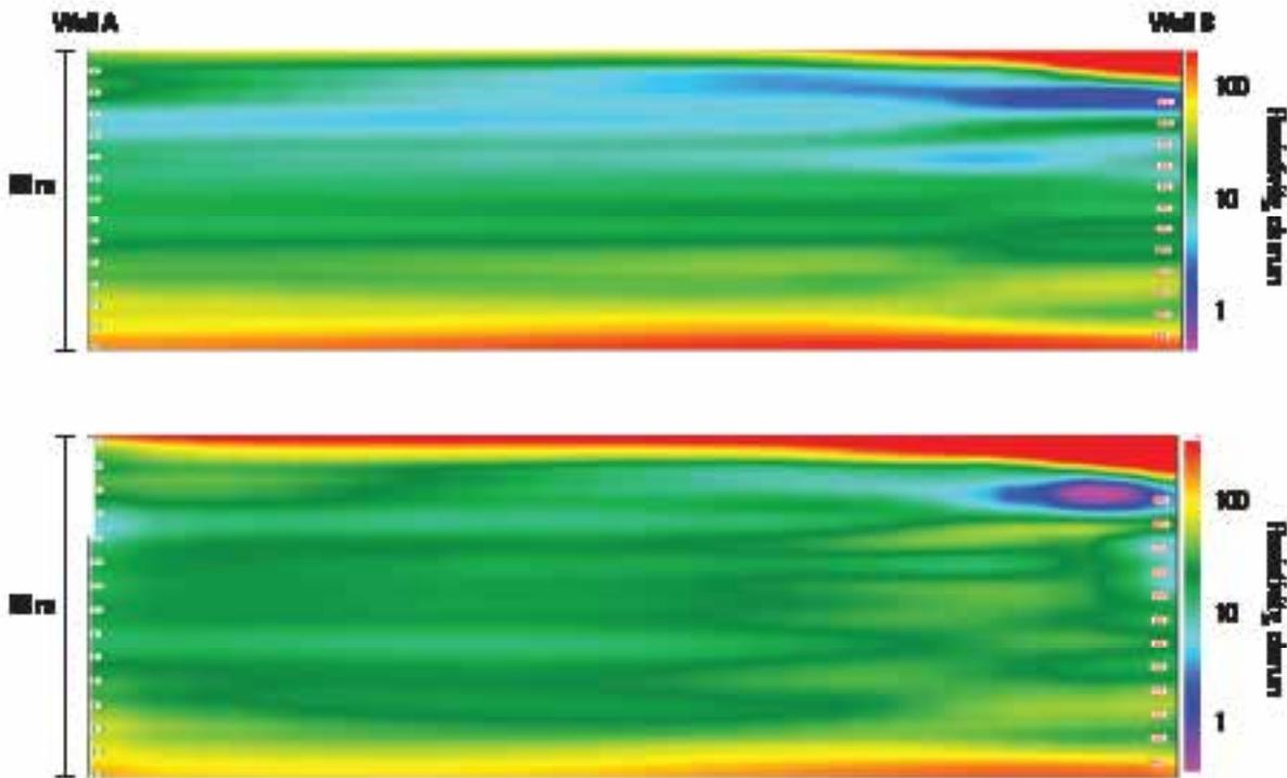
*In the top panel, the baseline model inferred from conventional resistivity logs indicates that the reservoir between the wells has watered out, with conductive injected fluid (blue) sweeping the reservoir. The inverted DeepLook-EM resistivity survey in the bottom panel indicates otherwise, with a higher resistivity range (green to yellow) in the same, high-porosity section of the reservoir.*
