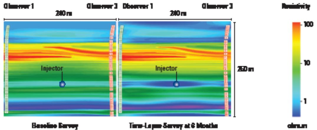
*Time-lapse DeepLook-EM crosswell resistivity surveys at a 6-month interval show a large water sweep preferentially from east to west between Wells 1 and 3.*
