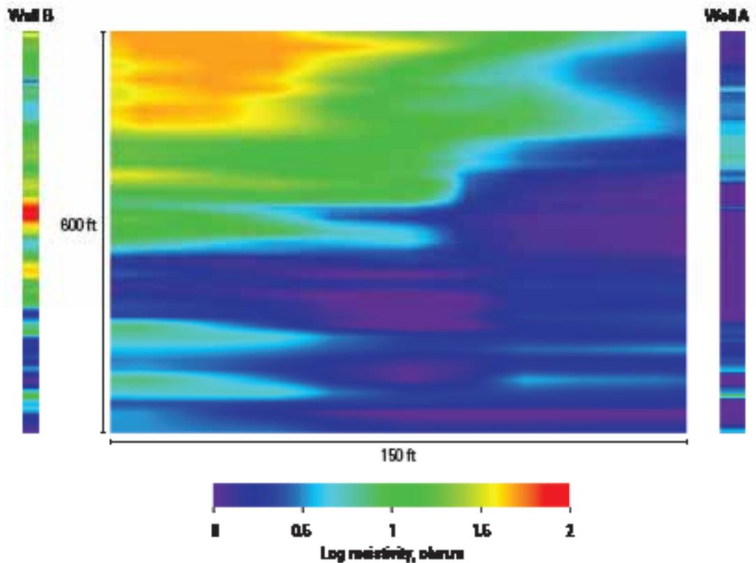
The DeepLook-EM resistivity profile between observation Wells B and A in the steamflooded San Joaquin field images an abrupt boundary midway, where the resistivity changes from 2 ohm.m in the depleted zone to more than 50 ohm.m.
