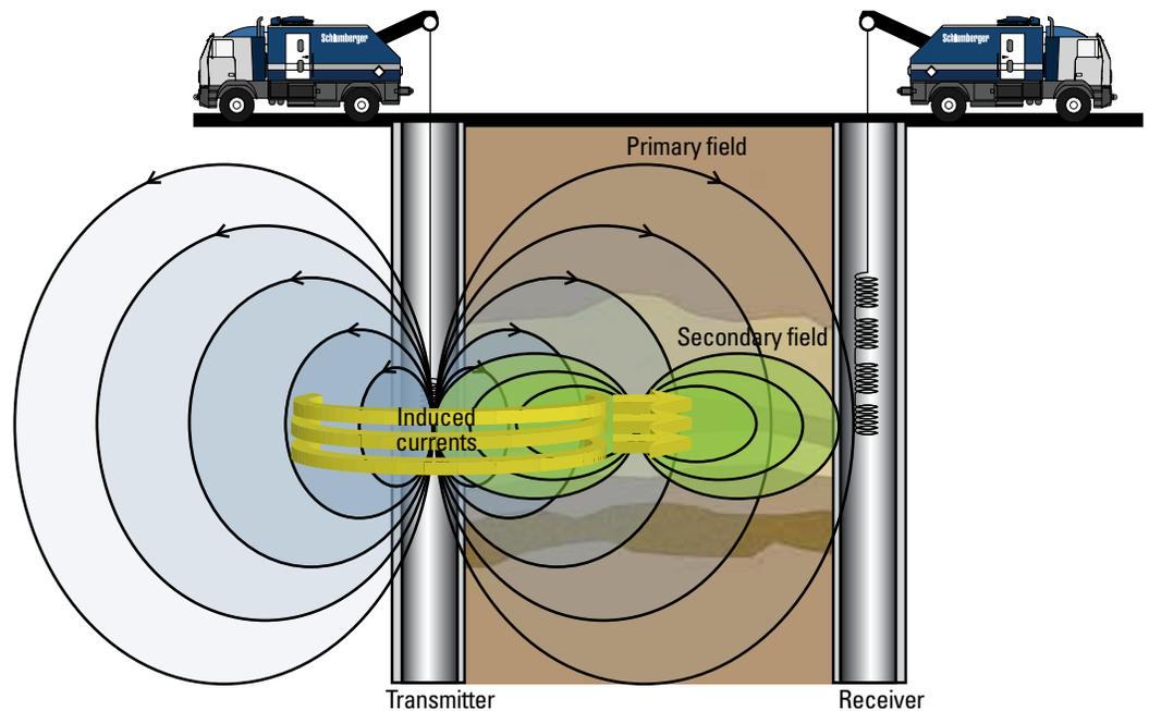
*Both the primary magnetic field generated by the transmitter and the secondary magnetic fields resulting from the induced currents are measured by the four receiver sensors.*
