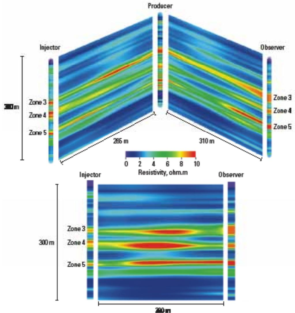
DeepLook-EM crosswell resistivity images between three wells in Gudao field show consistent, continuous producing zones, with the higher resistivity in Zone 5 indicating bypassed oil.
