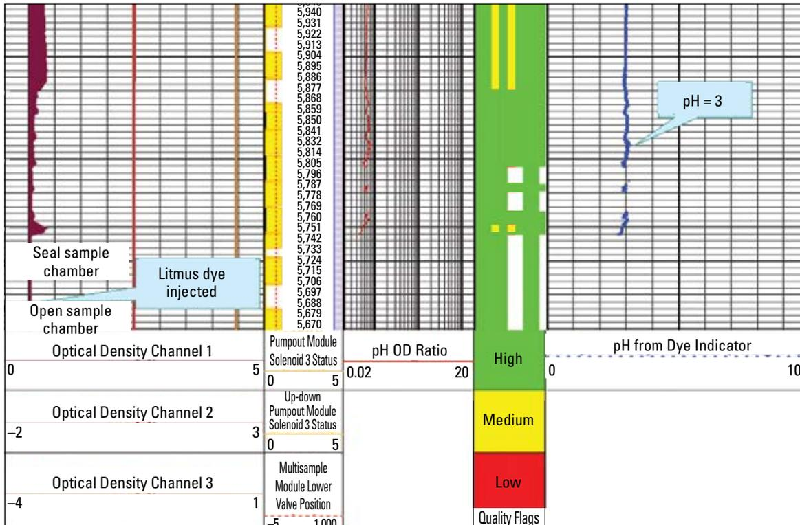
InSitu pH measurement of pH = 3 indicated high CO<sub>2</sub> that was missed in laboratory analysis conducted after the sample was flashed. With knowledge of the actual CO<sub>2</sub> content, the operator could minimize subsequent corrosion and scaling problems.
