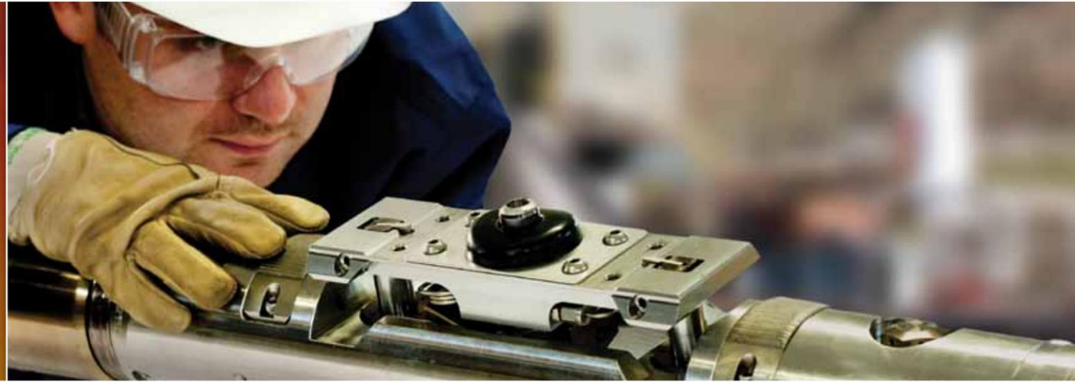
Each PressureXpress-HT tool is subjected to pressure-temperature cycling in test wells at the manufacturing center before deployment for field operations.
