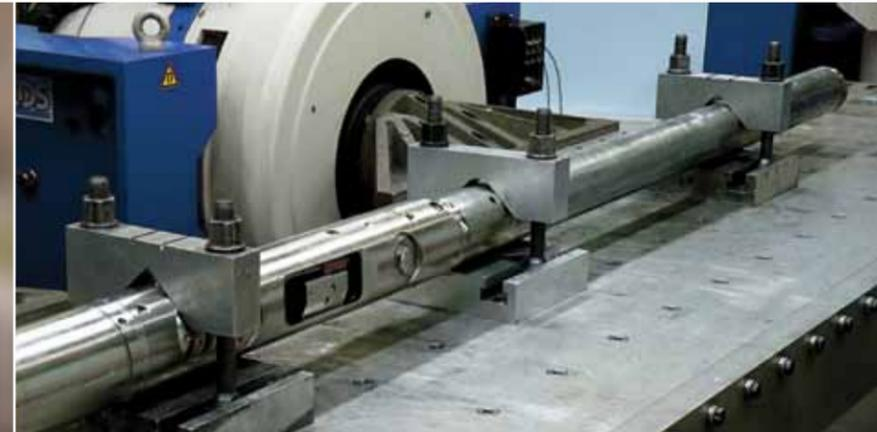
Shock and vibration testing of PressureXpress-HT tools is conducted using specially designed equipment.
