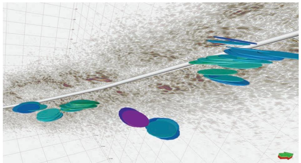
The 3D STC reflector discs imaging the dip and azimuth are shown with the migrated monopole image along the wellbore.
