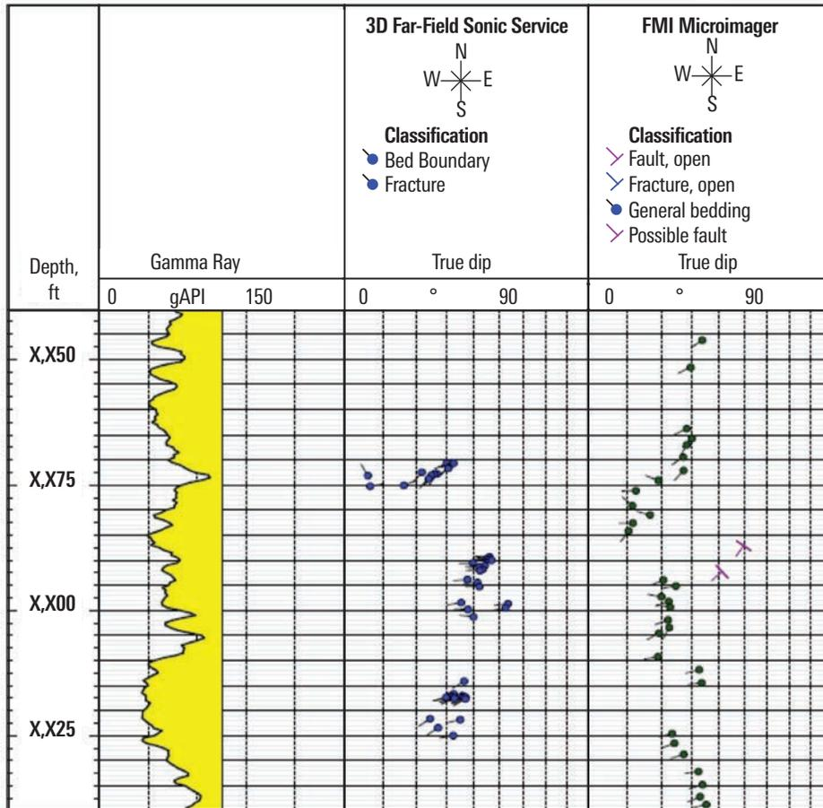
Dip and azimuth from 3D sonic imaging in Track 3 confirm far-field structural changes interpreted in Track 2 from the FMI microimager above and below the fault identified at about X,X85–X,X95 ft.
