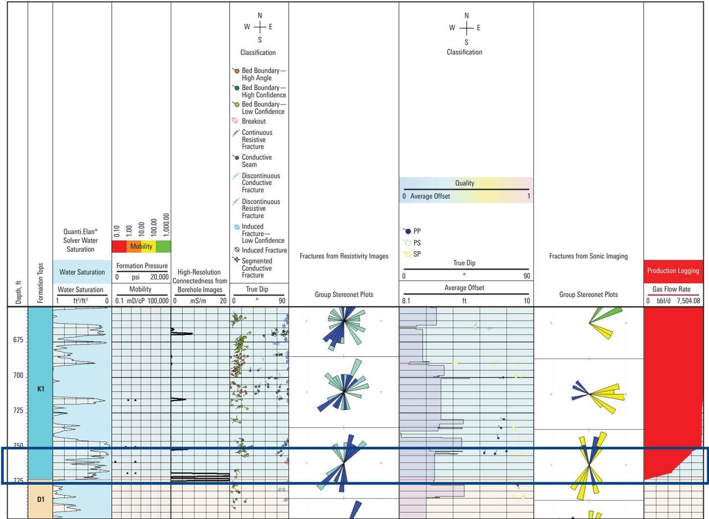
As shown in the processed data displayed in the Techlog\* wellbore software platform, 3D far-field sonic service quantified that the natural fractures in the high-productivity zone (blue box) are more directionally consistent from the near- to the far-field reservoir, as compared with the larger zones above.
