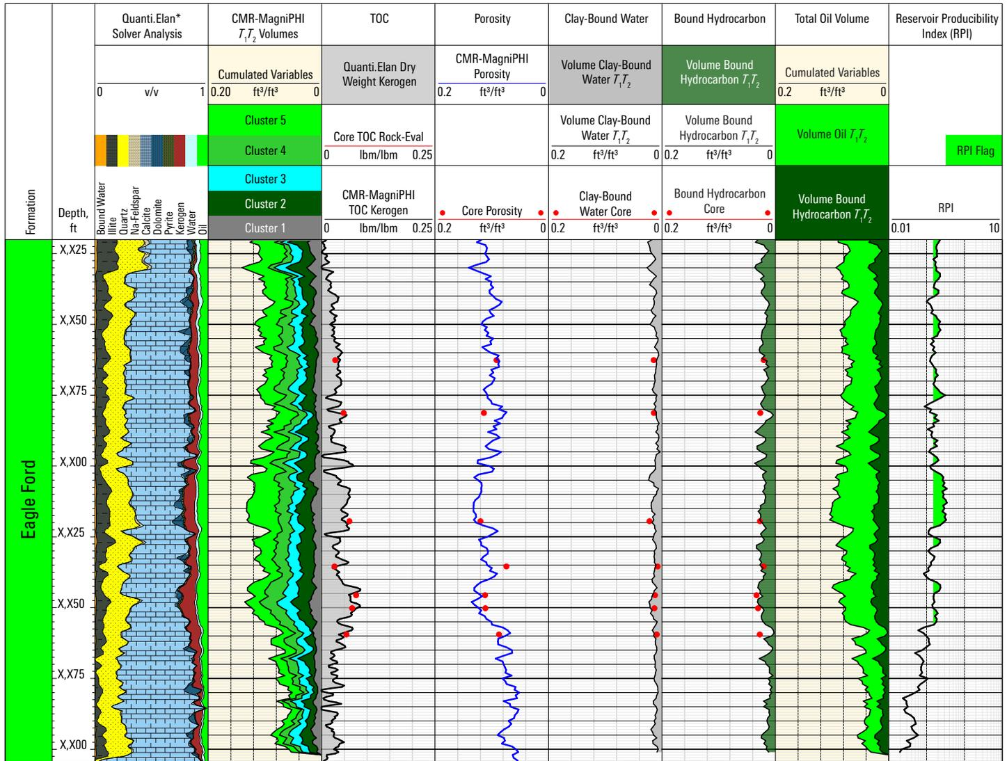
The petrophysical model for this Eagle Ford well was developed using measurements from CMR-MagniPHI and Litho Scanner services and traditional triple-combo logging. The results are in good agreement with those from core analysis. The refined reservoir volumetrics identify potential landing targets on the basis of the reservoir productivity index and permeability from the CMR-MagniPHI service.
