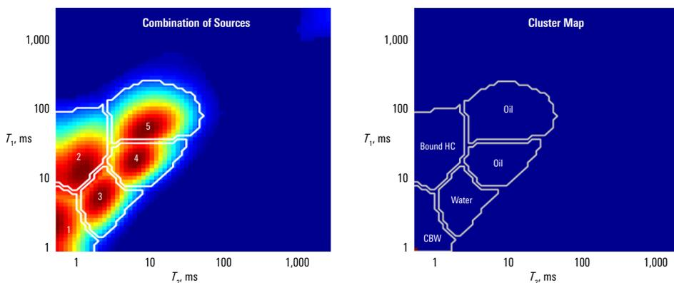
Mapping of continuously acquired  $T_1T_2$  obtained with CMR-MagniPHI service over a 195-ft interval reveals the complex distribution of fluids within the Eagle Ford Formation.
