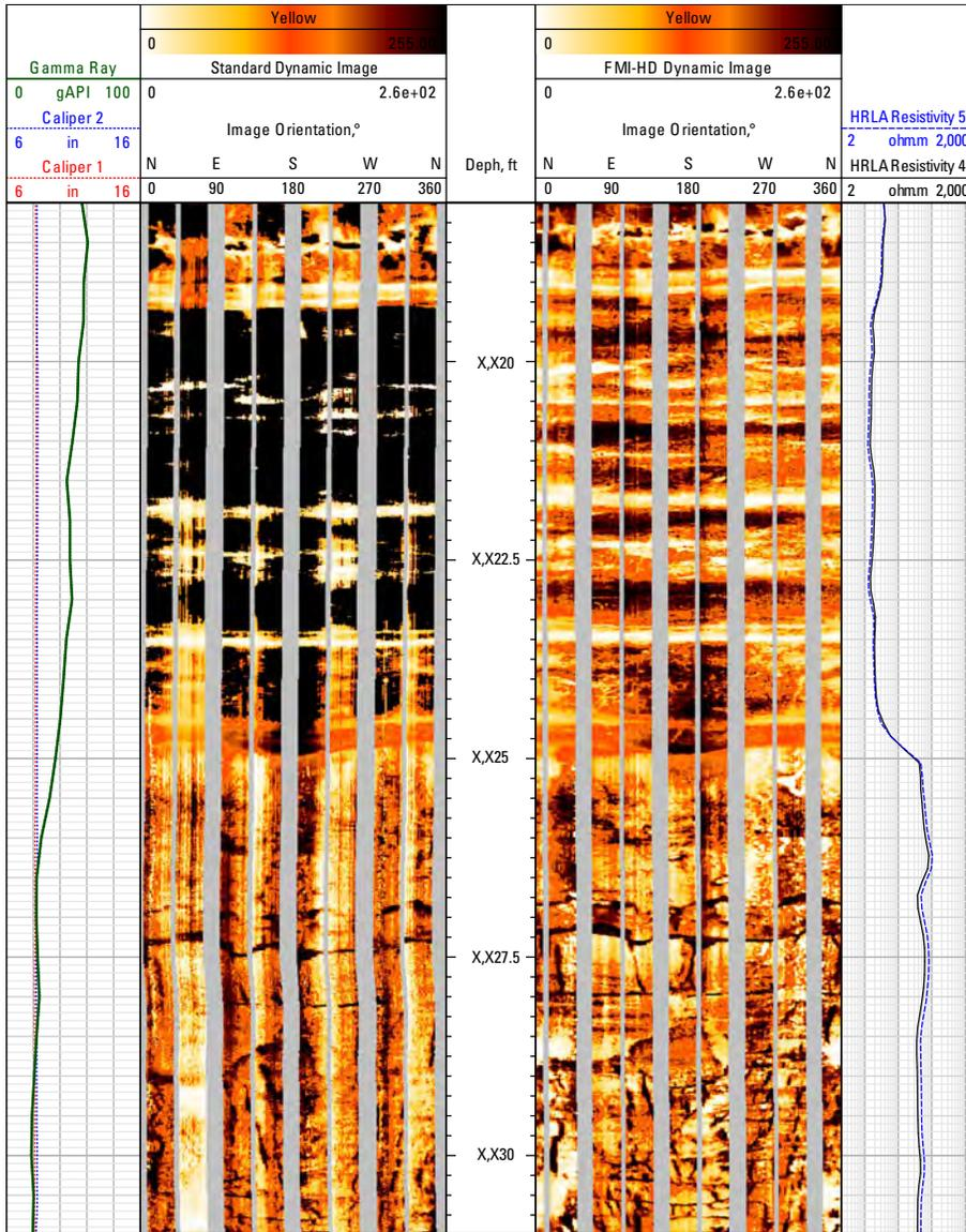
Where the formation resistivity was highly variable, only the FMI-HD microimager optimally captured both high- and low-resistivity formation images in a single pass. Automatic signal processing optimization adjusted the FMI-HD microimager to image the entire dynamic range of formation resistivity, whereas the conventional tool had to be retrieved and reset by the engineer to optimize it for either high- or low-resistivity formations and then the well relogged.
