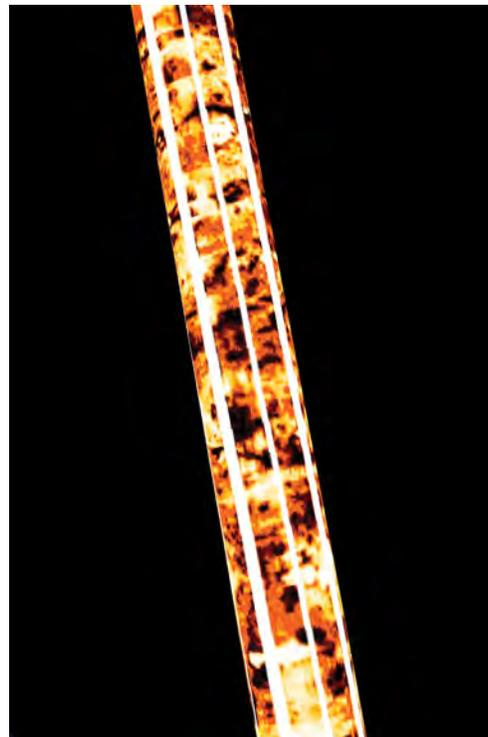
*The images at 0.2-in vertical resolution from the FMI-HD microimager can be displayed on a virtual 3D core by the Techlog\* wellbore software platform at any scale down to 1:1. Patches of well-developed vuggy porosity are clearly visible as dark spots in this example.*
