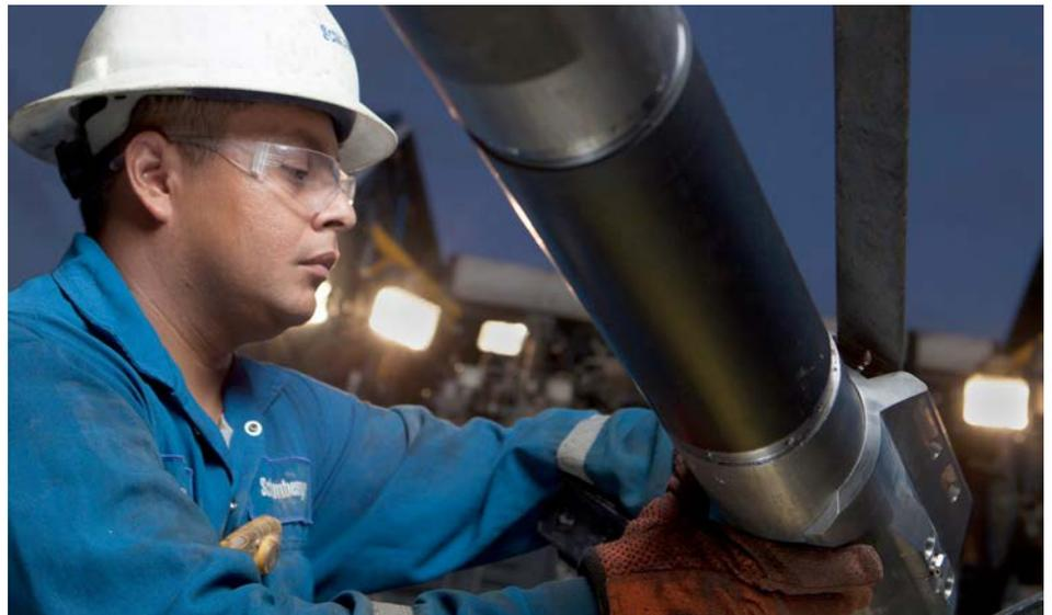
*Litho Scanner service employs a sourceless pulsed neutron generator to accurately measure an expanded set of elements compared with conventional spectroscopy tools.*
