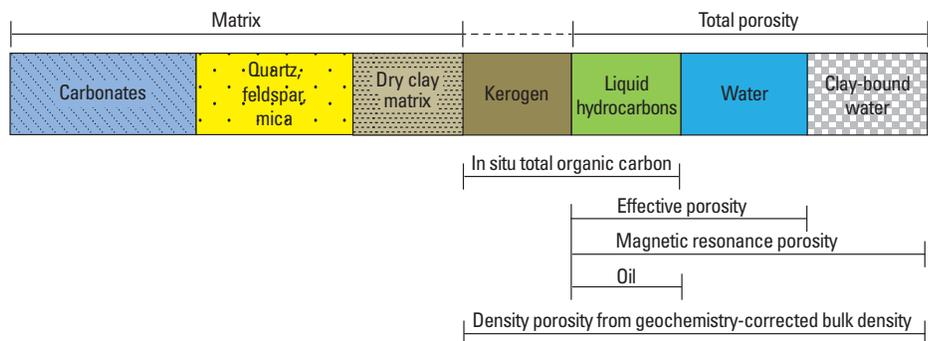
*Litho Scanner spectroscopy service accurately quantifies all the dry-weight components of the matrix and delivers a stand-alone in situ determination of TOC, which incorporates the reservoir contents for kerogen and liquid hydrocarbon. The CMR-Plus magnetic resonance measurement sees all the fluids and is not influenced by kerogen. This difference in measurement enables easily dividing the TOC into kerogen and liquid contents.*
